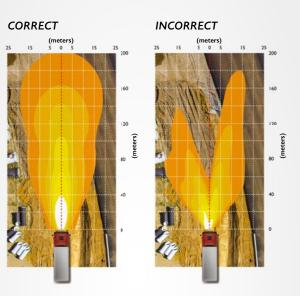
Off-road illumination. To ensure optimum visibility when working with your headlamps on, your headlamps need to be positioned correctly such as to provide an intense and precise source of luminous power – this is the only way to guarantee your comfort and safety while also taking the stress out of driving.
