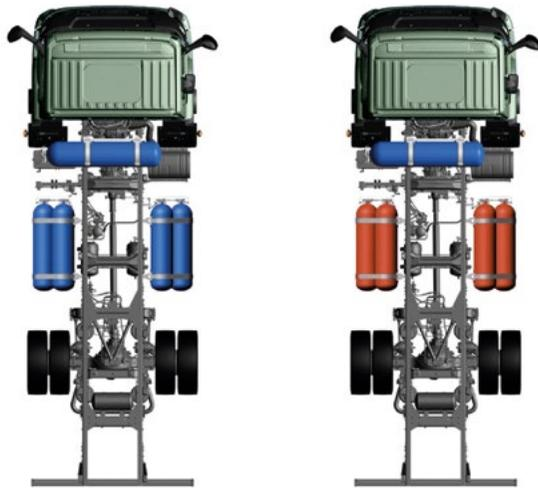
Tanks on both sides and behind cab
